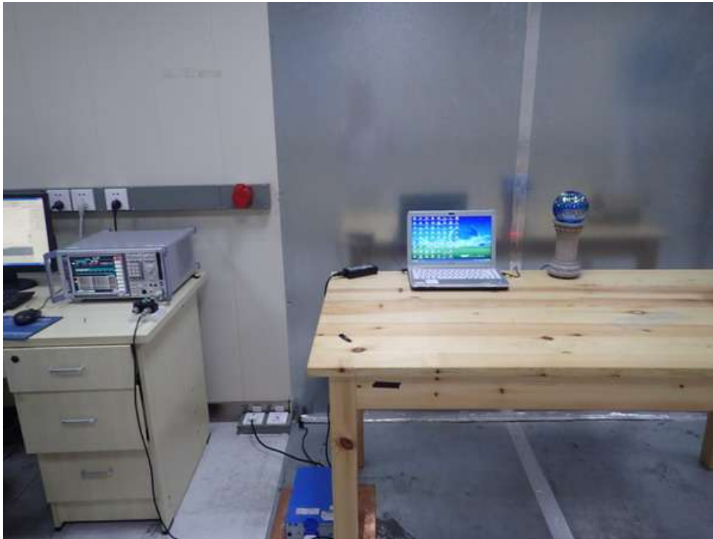
FCC RADIATED EMISSION TEST SETUP
