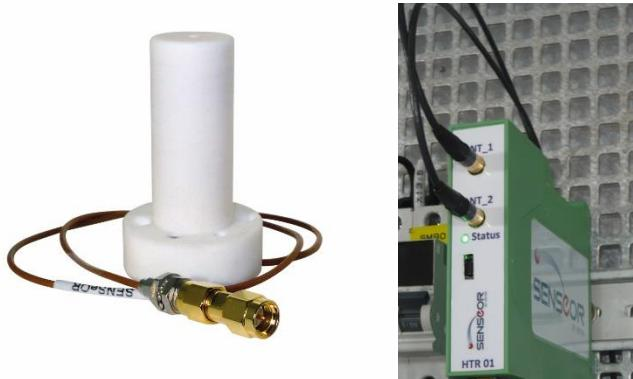
One antenna on “Ant\_1A” is needed in TS6 for interrogation of six sensors in “free-air”.
