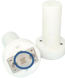
If you are using a reference sensor, make sure that the sensitive element of this sensor will be placed as close as possible to the SAW temperature chip, but not in contact with it.
