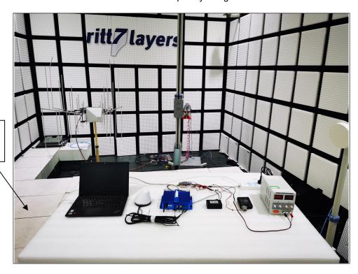
the absorbing material is under the foam
