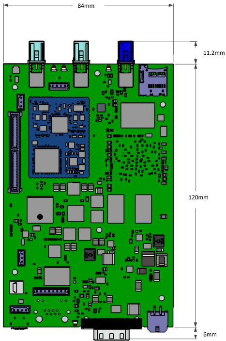
FIGURE 3 - PCB DIMENSIONS WITH MOUNTING HOLE LOCATIONS
