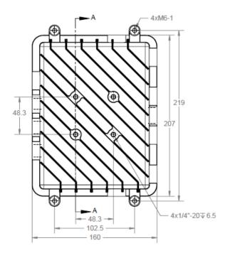
FIGURE 8 - XBU ENCLOSURE MOUNTING HOLE
