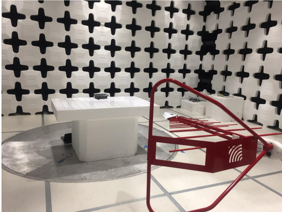
Radiated Emissions Below 1GHz setup – Front
