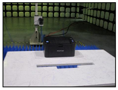
1.2 CONDUCTED EMISSION TEST SETUP
