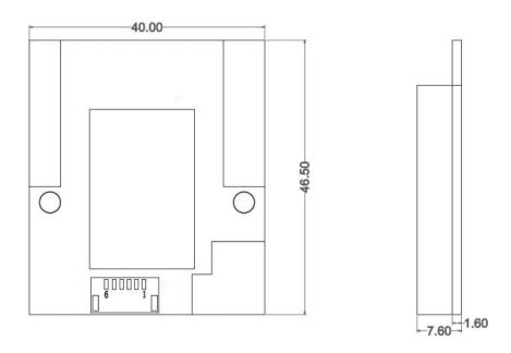
Module dimension: 46.5mm\*40.0mm\*7.6mm (L\*W\*H; Tolerance: ±0.15mm)
