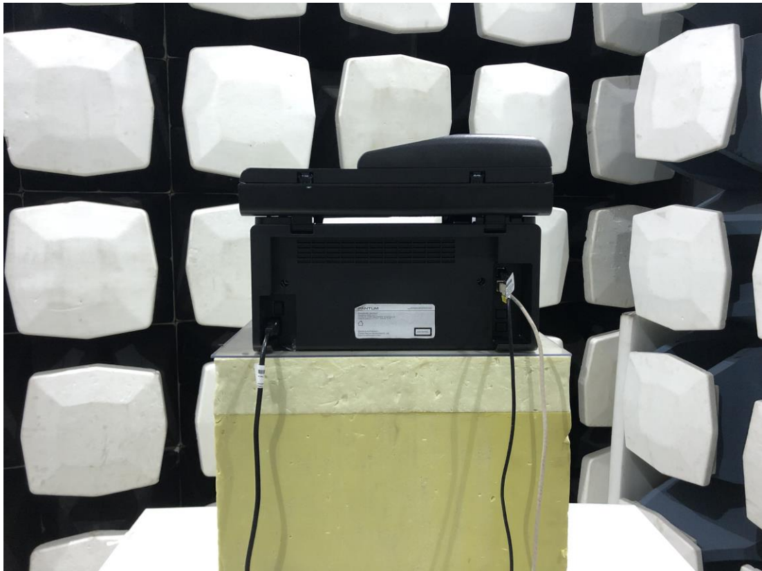
The EUT and transmitting antenna was centered on the turntable.
