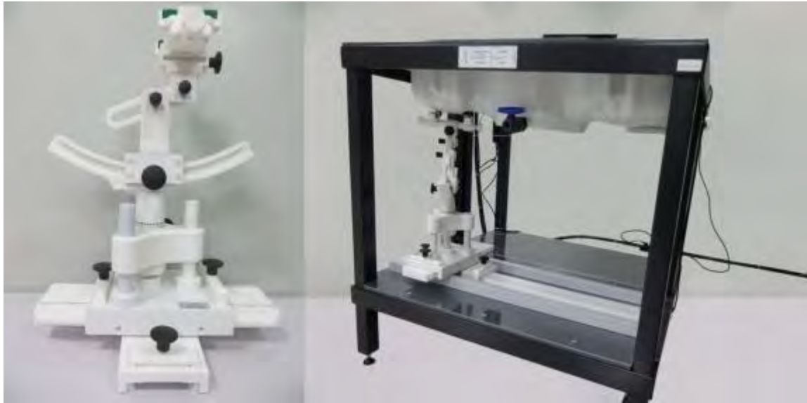
Device holder supplied by SATIMO
