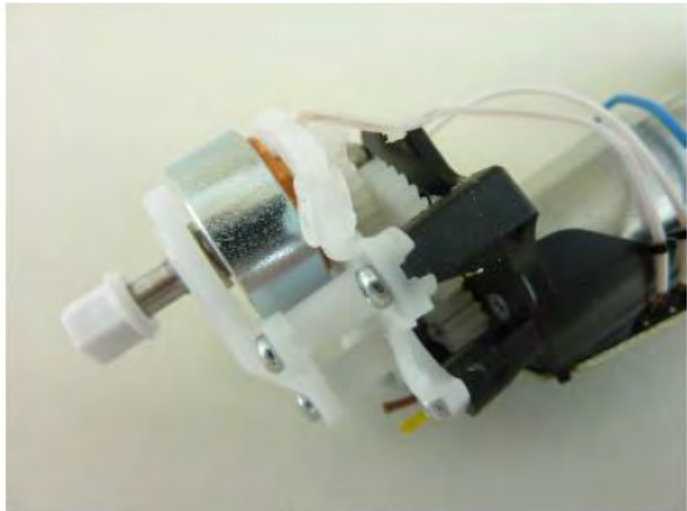
Figure 1: Custom-built flow control device.
