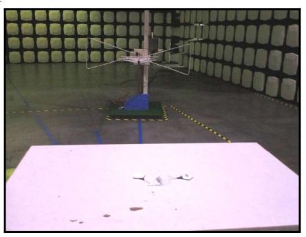
Above 1GHz: (full anechoic chamber)
