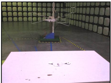
Above 1GHz: (full anechoic chamber)
