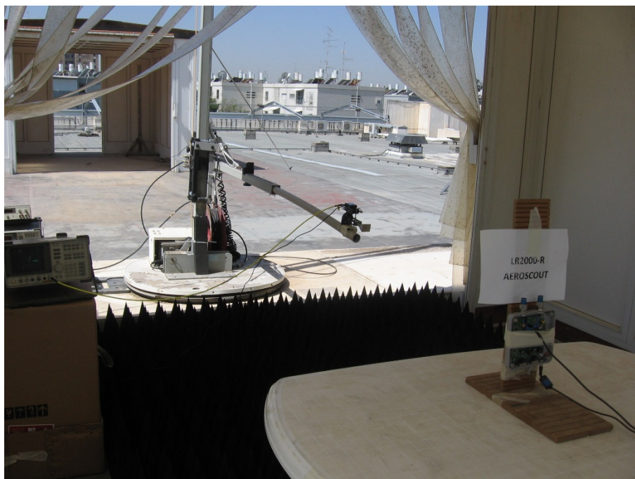
Figure 9. Radiated Emission Test Setup - 26.5 GHz-40 GHz
