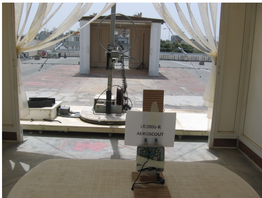
Figure 5. Radiated Emission Test Setup
