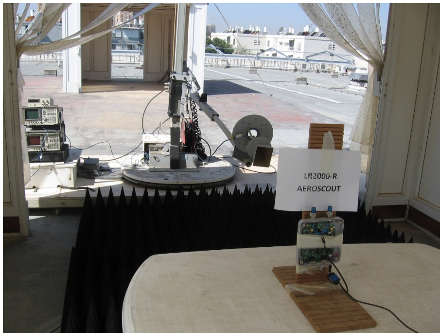
Figure 8. Radiated Emission Test Setup – 18 GHz -26.5 GHz
