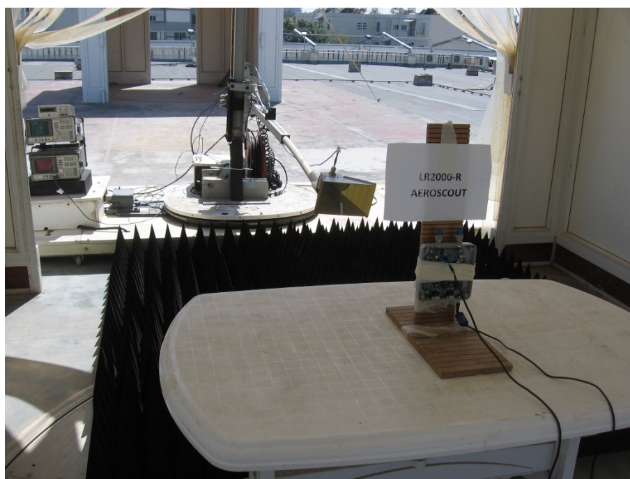
Figure 7. Radiated Emission Test Setup – 1 GHz – 18 GHz
