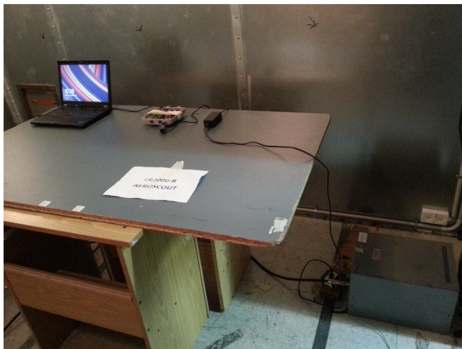
Figure 4. Conducted Emission Test Setup
