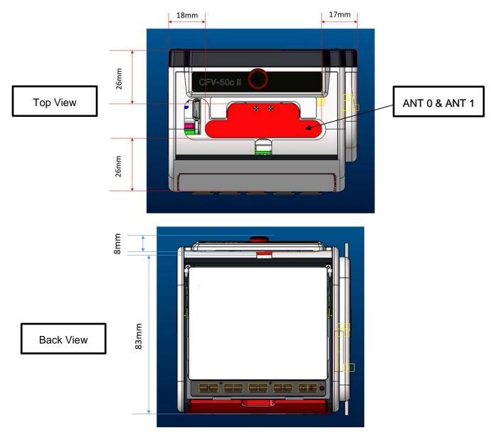
Per FCC KDB 941225D07: UMPC mini-tablet devices must be tested for 1-g SAR on all surfaces and side edges with a transmitting antenna located at  $\leq$  25 mm from that surface or edge.
