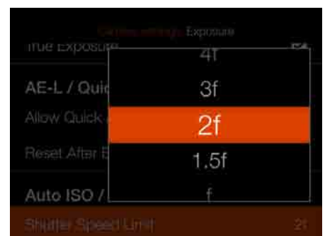
Shutter speed limit setting as a function of focal length.
