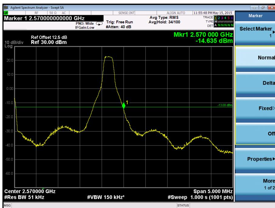
**Band Edge on Configuration QPSK-5M / 25RB Channel
