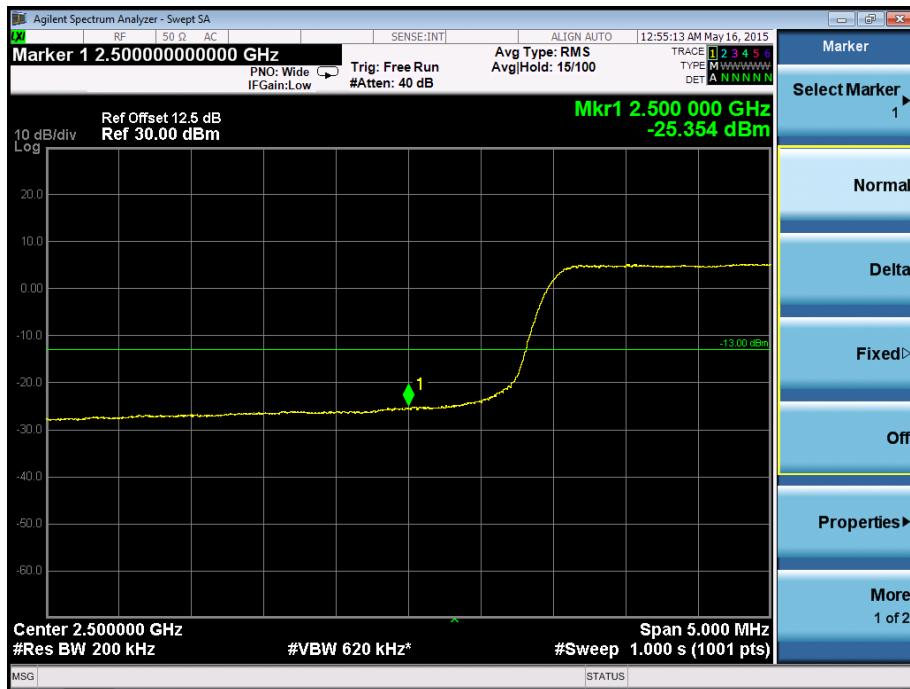
**Band Edge on Configuration 16-QAM-20M / 100RB Channel
