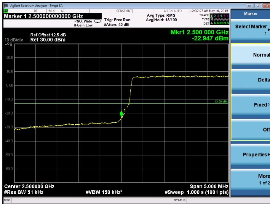
**Band Edge on Configuration 16-QAM -5M / 25RB Channel
