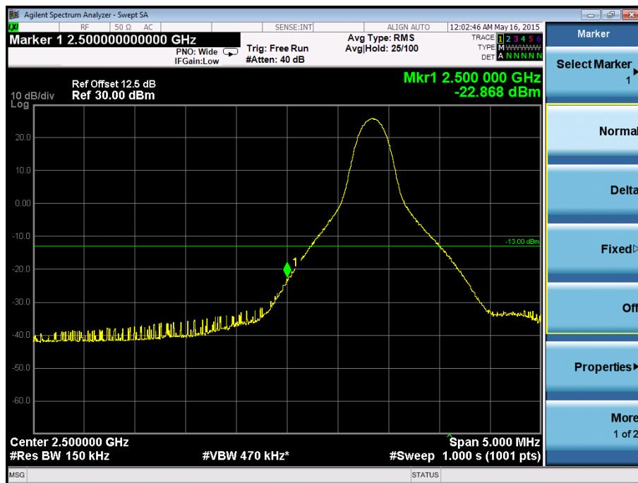
**Band Edge on Configuration QPSK-15M / 1RB Channel**
