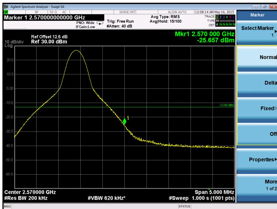
**Band Edge on Configuration QPSK-20M / 100RB Channel
