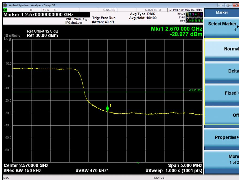
**Band Edge on Configuration 16-QAM-20M / 1RB Channel
