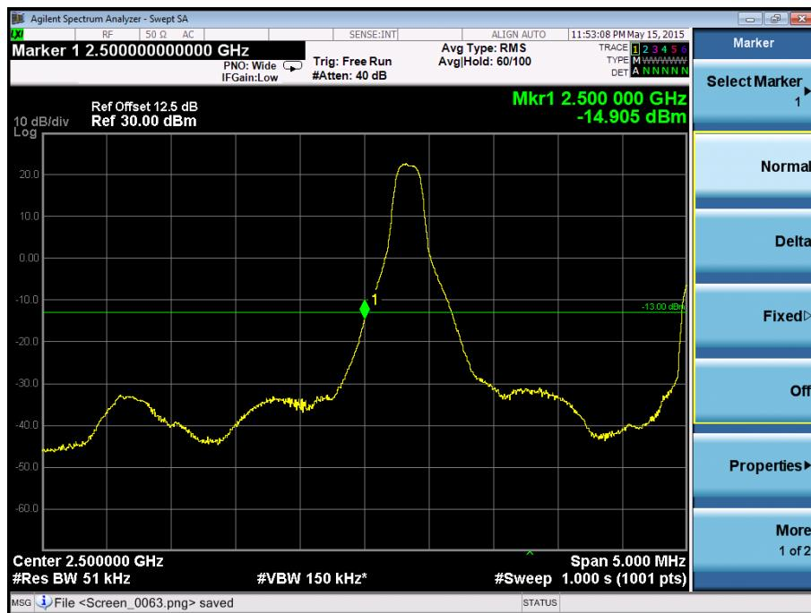
**Band Edge on Configuration QPSK-5M / 1RB Channel
