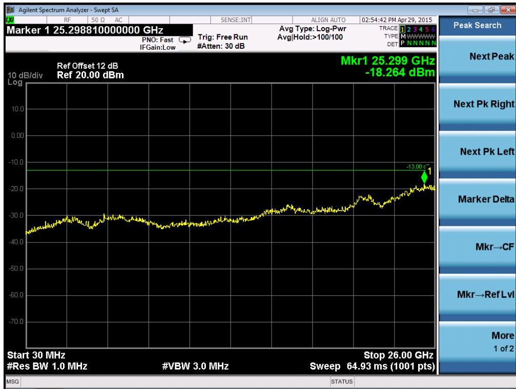
**Conducted Spurious of Configuration-QPSK-5M/1RB channel Highest**
