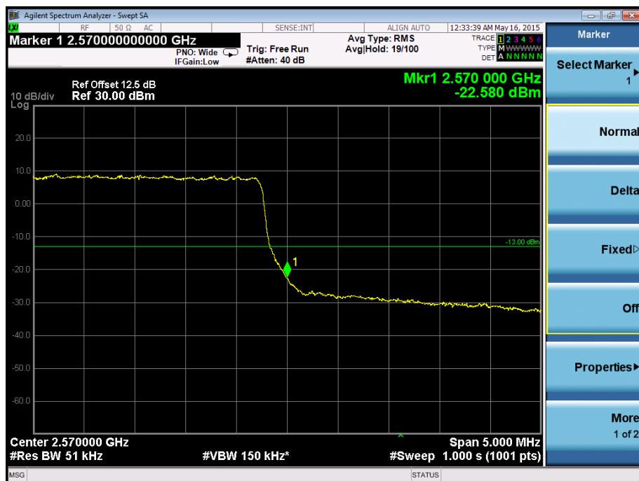
**Band Edge on Configuration QPSK-10M / 1RB Channel
