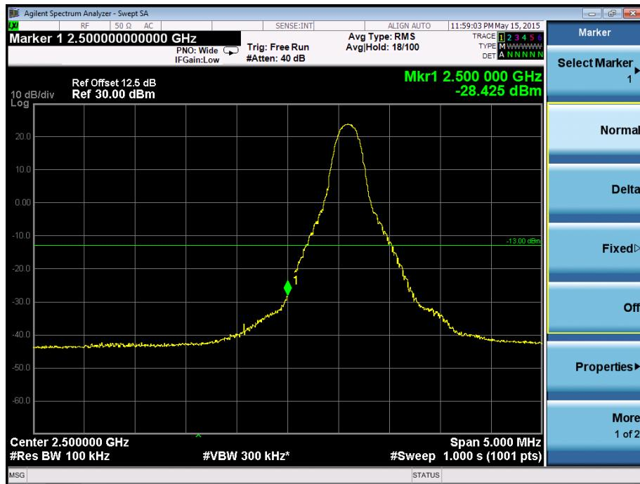
**Band Edge on Configuration 16-QAM-10M / 1RB Channel**
