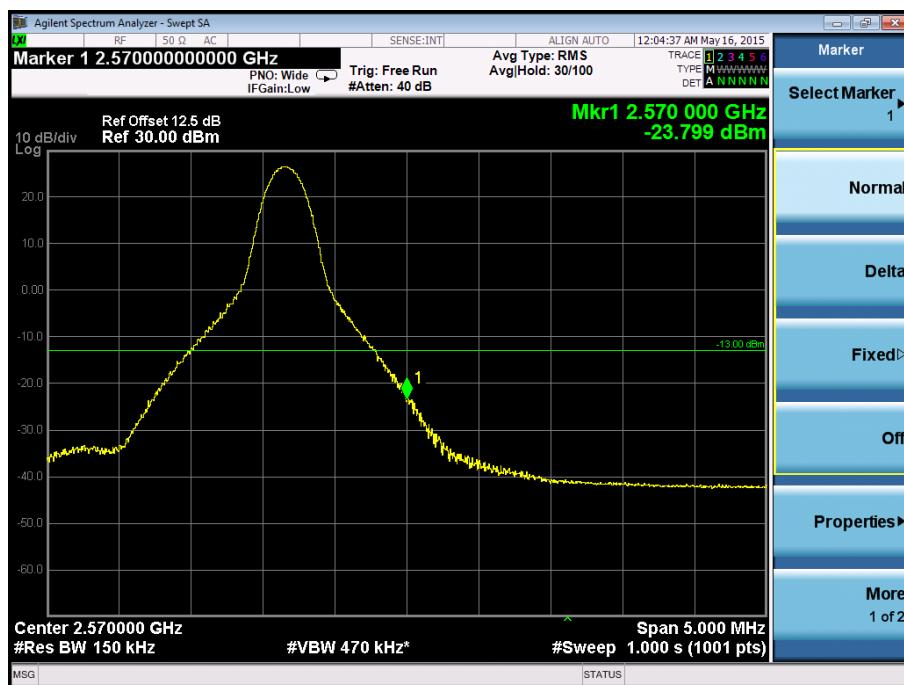
**Band Edge on Configuration QPSK-15M / 75RB Channel
