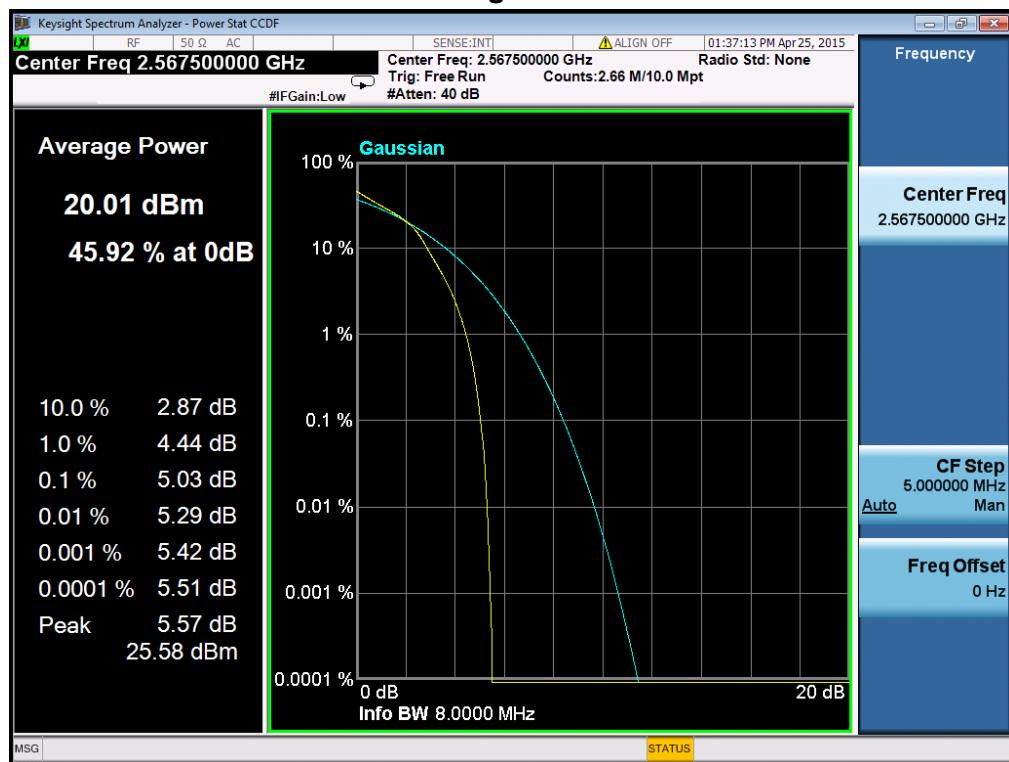
**Peak to Average Radio of Configuration-16-QAM-10M/1RB channel**
