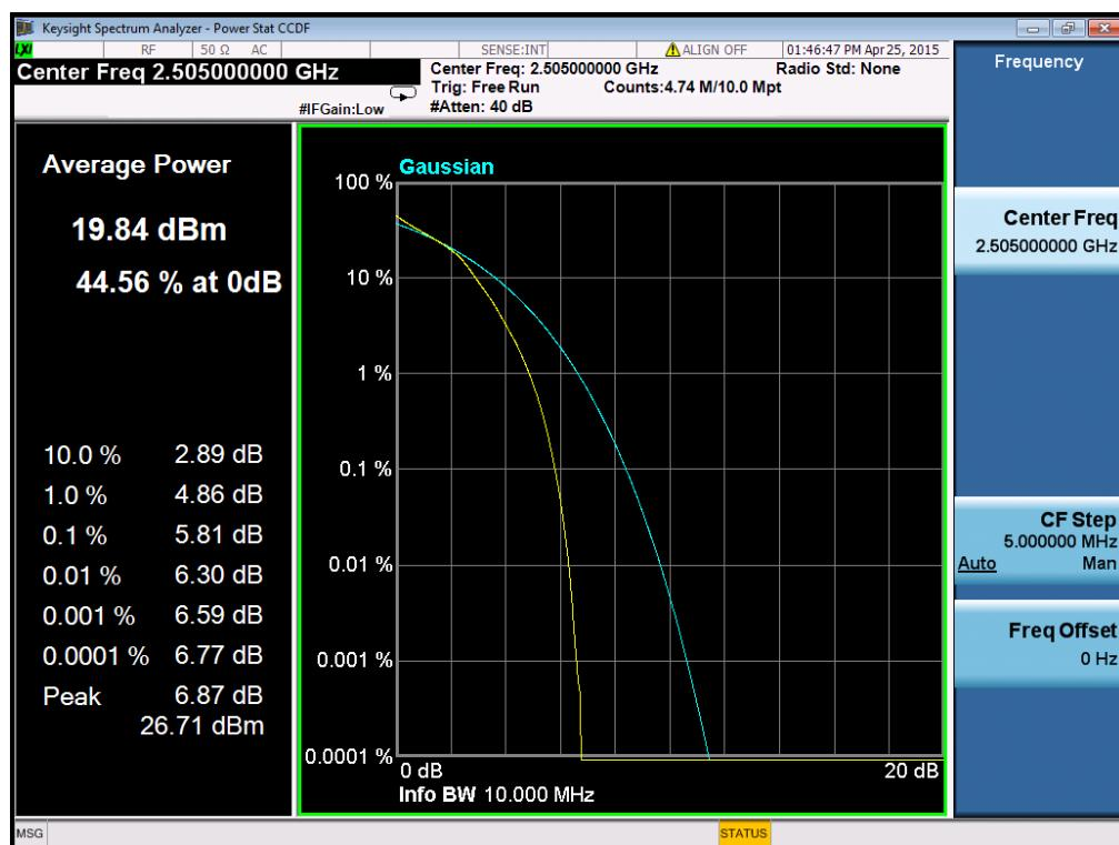
**Peak to Average Radio of Configuration-16-QAM-10M/1RB channel**
