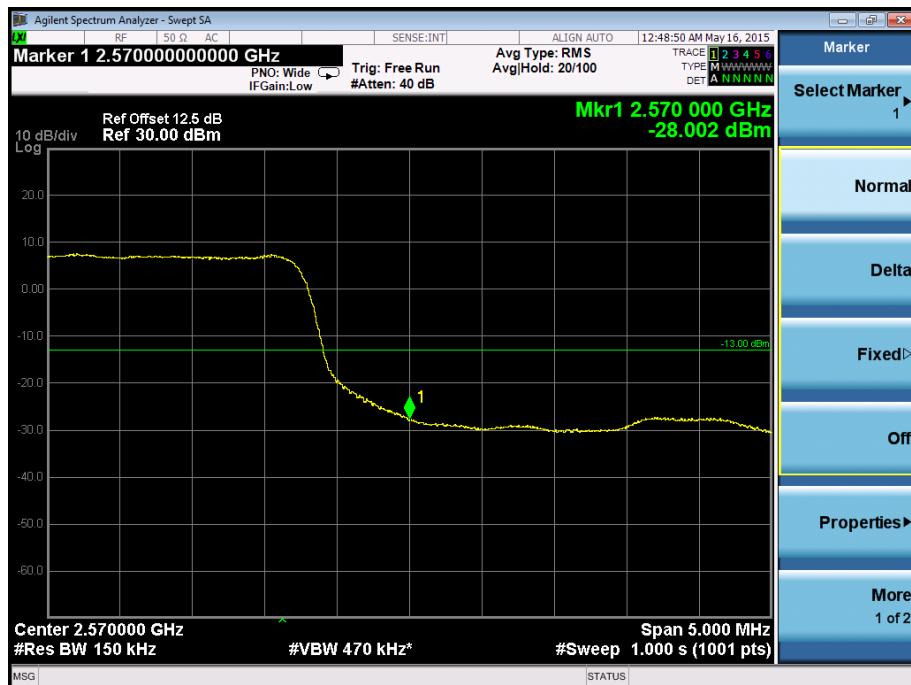
**Band Edge on Configuration QPSK-20M / 1RB Channel**
