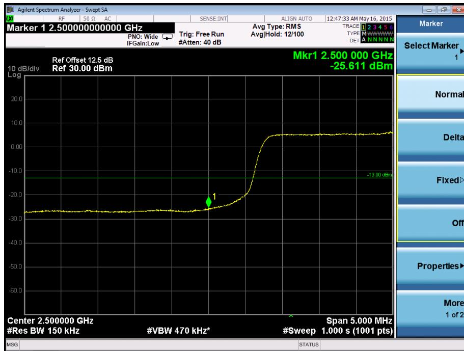
**Band Edge on Configuration Q16-QAM-15M / 75RB Channel
