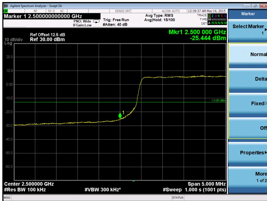
**Band Edge on Configuration 16-QAM-10M / 50RB Channel**
