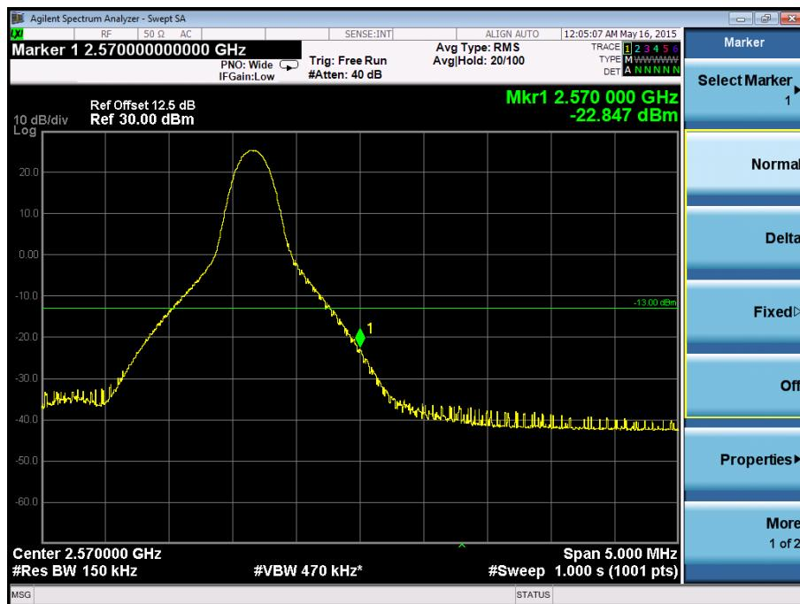
**Band Edge on Configuration 16-QAM-15M / 75RB Channel
