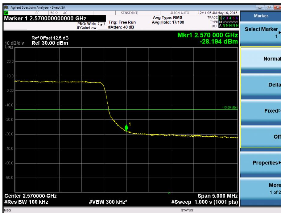
**Band Edge on Configuration 16-QAM-15M / 1RB Channel
