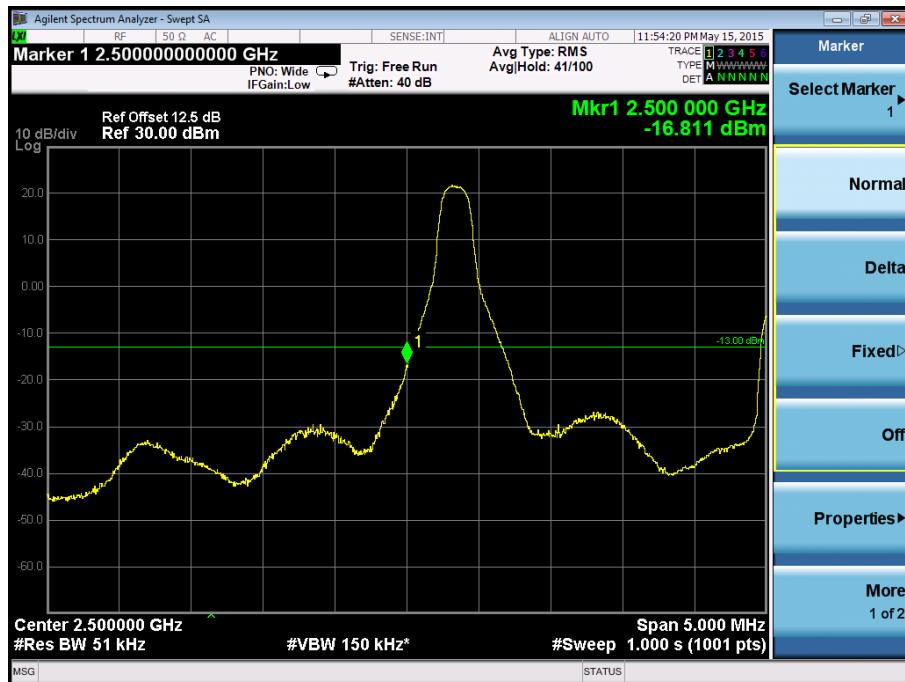
**Band Edge on Configuration 16-QAM -5M / 1RB Channel**
