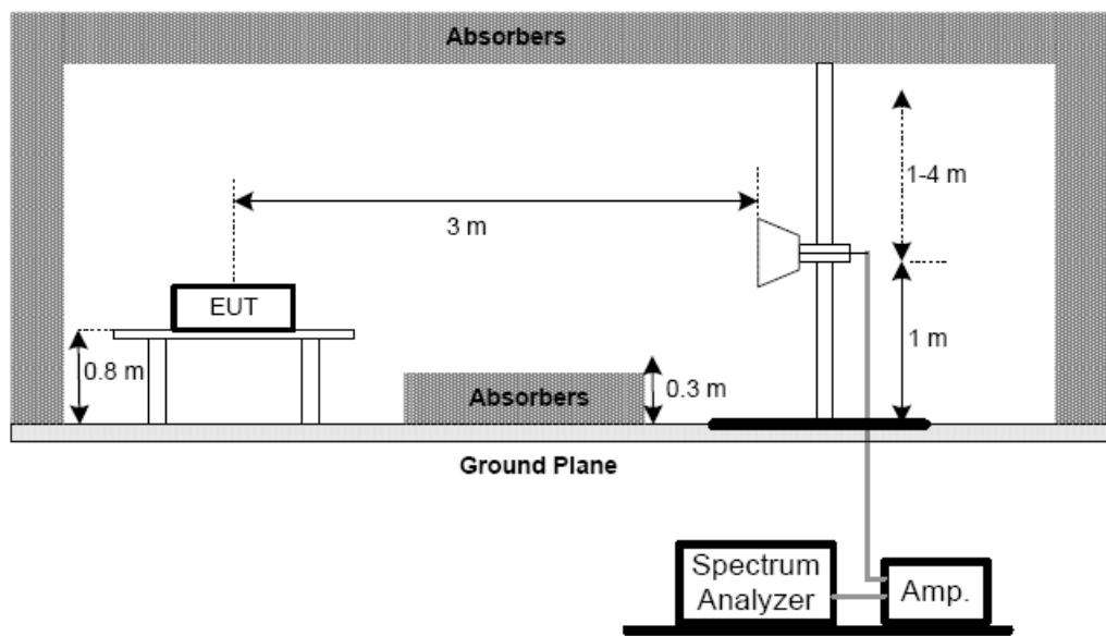
(C) For radiated emissions below 30MHz
