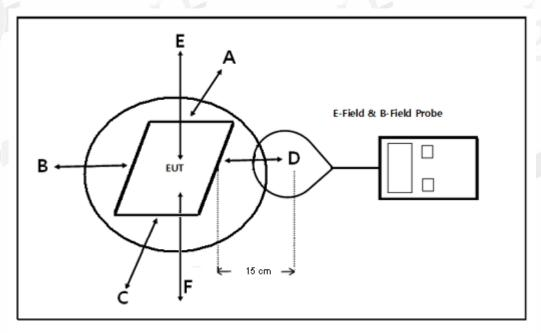
Note: Due to installation limitations no tests from the underside of the charging device (Test Position F) are required. The test position F is required when the distance is 0cm.
