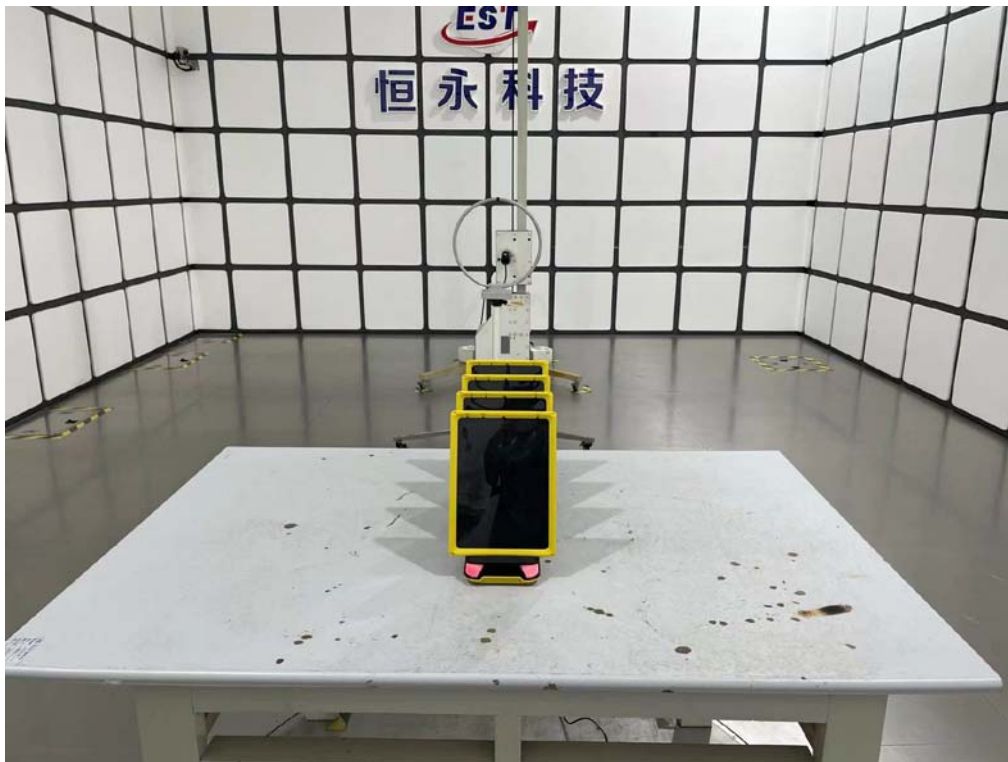
Radiated emission test: Below 30MHz
