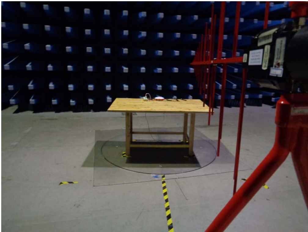
Radiated Spurious Emissions Test Setup Below 1GHz
