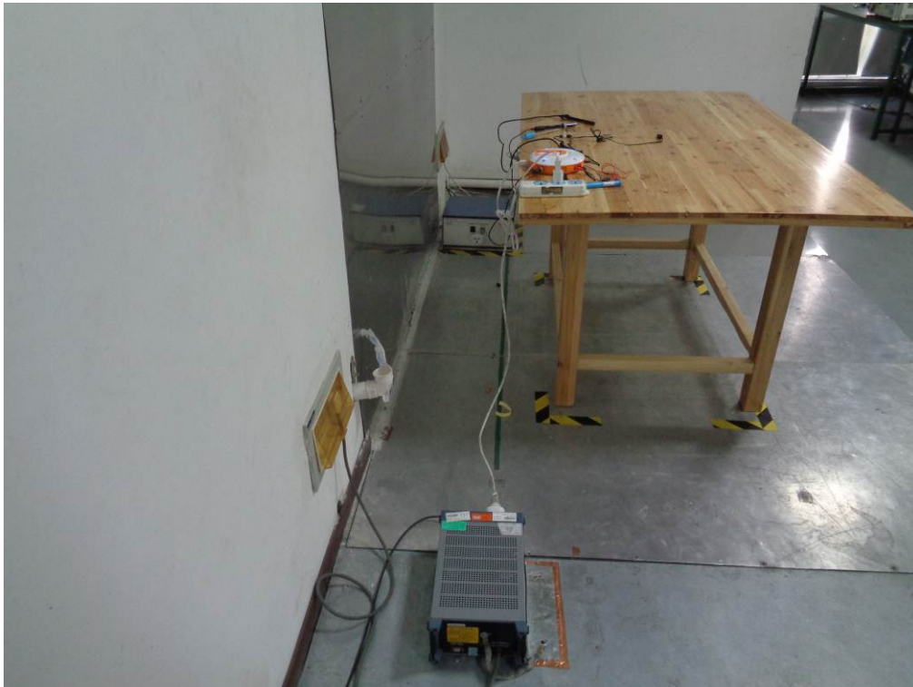
Conducted Emissions Test Setup – Side View
