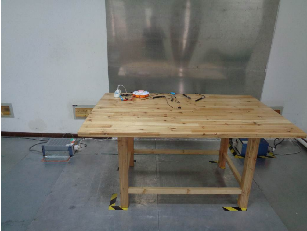
Conducted Emissions Test Setup – Front View
