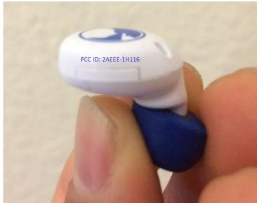
However, we had wrongly believed the size that 4 point font would equate to the text size in the image above. However, text at the length of our FCC ID would cause 4 point font would be 22mm in width, whereas the above image has the font at a 9.4mm width.
