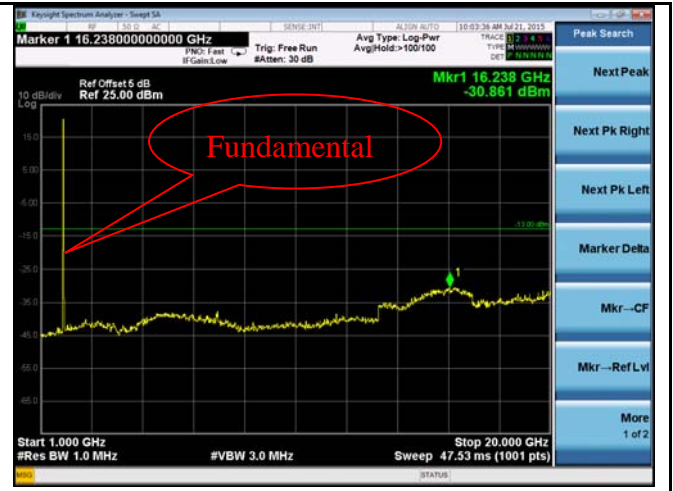
LTE band 2 – Low CH Above 1GHz QPSK
