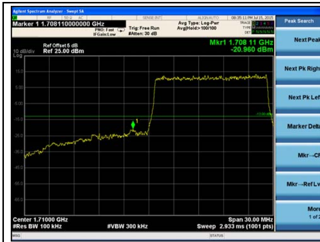
LTE Band 4 - Low Channel 16QAM-15
