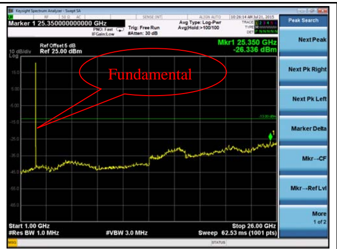
LTE band 7 – Low CH Above 1GHz 16QAM
