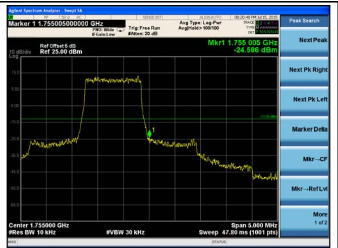
LTE Band 4 - High Channel QPSK-1.4
