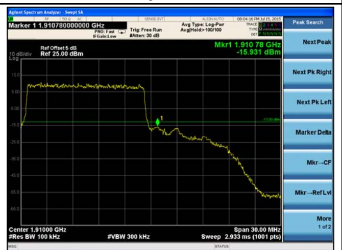
LTE Band 2 - High Channel QPSK-15
