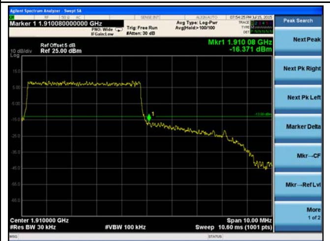
LTE Band 2 - High Channel QPSK-5
