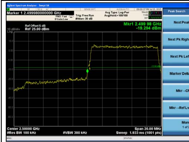
LTE Band 7 - Low Channel QPSK-10
