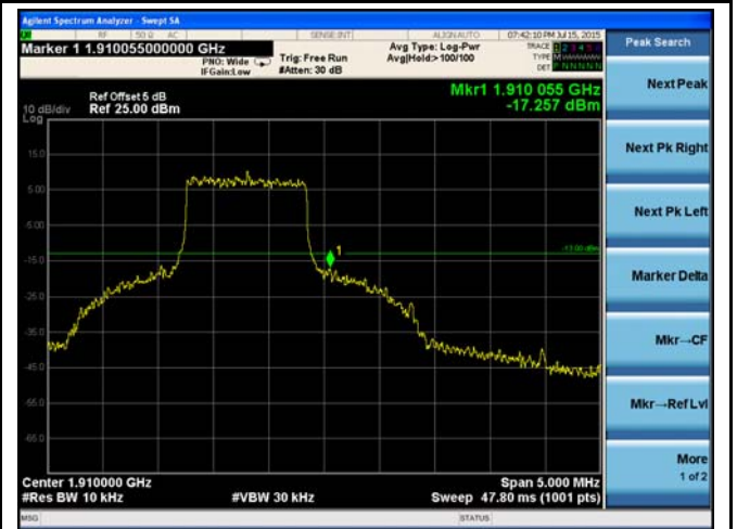
LTE Band 2 - High Channel 16QAM-1.4
