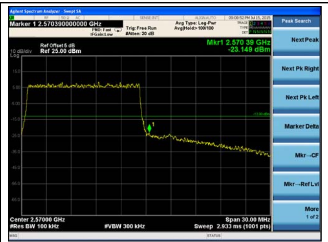
LTE Band 4 - High Channel 16QAM-15
