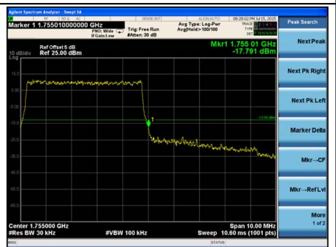
LTE Band 4 - High Channel 16QAM-5
