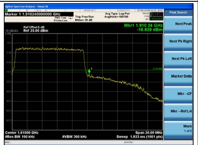
LTE Band 2 - High Channel 16QAM-10
