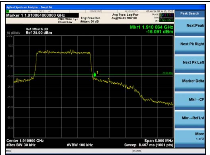
LTE Band 2 - High Channel 16QAM-3
