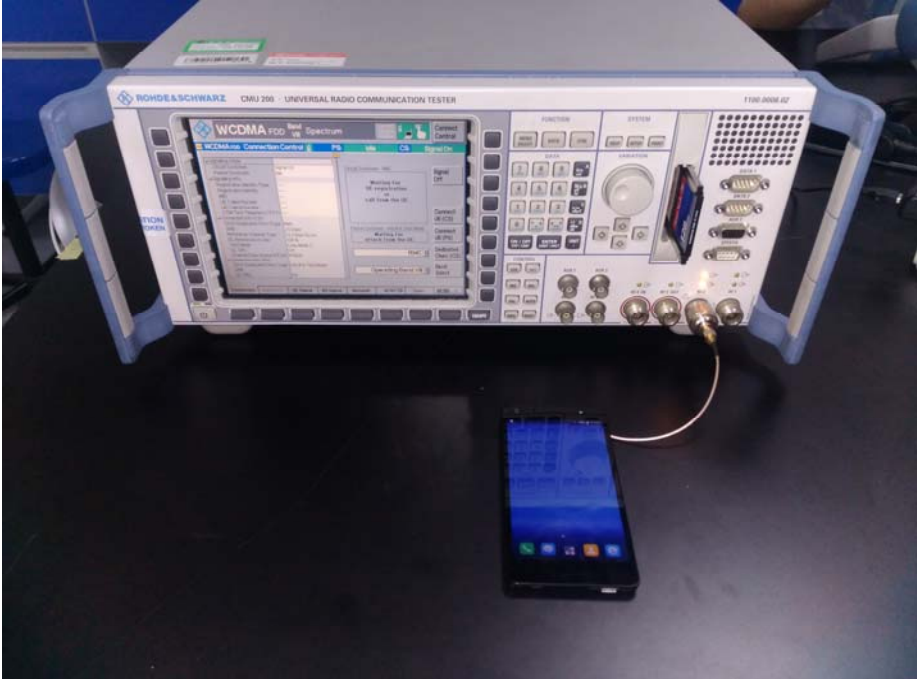
Photograph –2G&3G Conducted Test Setup
