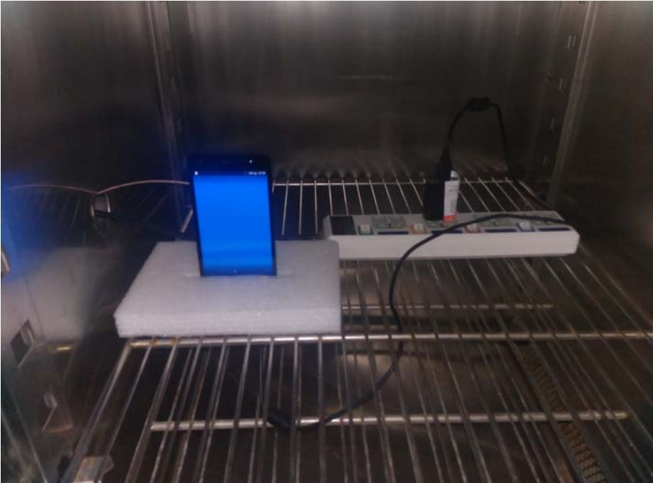
Photograph – Extreme Condition Test Setup
