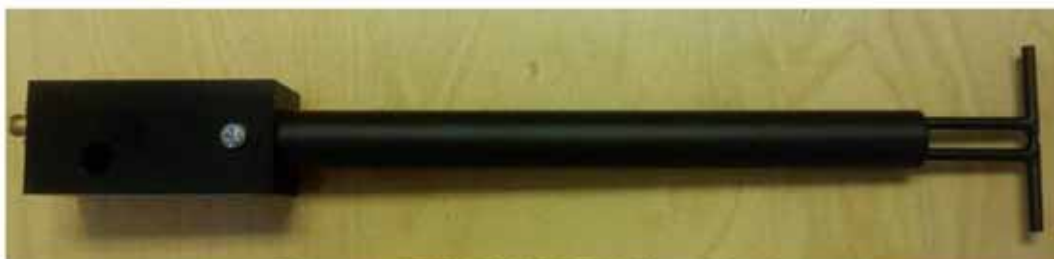
Figure 1 – MVG COMOSAR Validation Dipole
