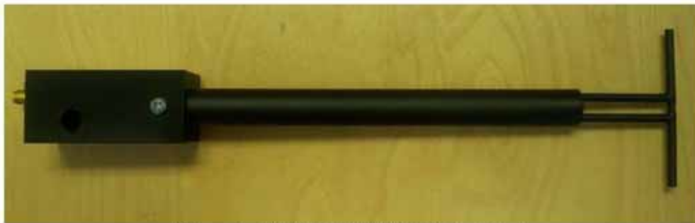
Figure 1 – MVG COMOSAR Validation Dipole
