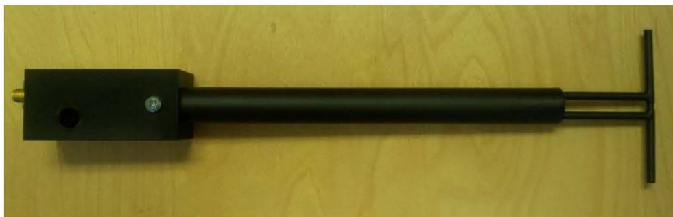
Figure 1 – MVG COMOSAR Validation Dipole
