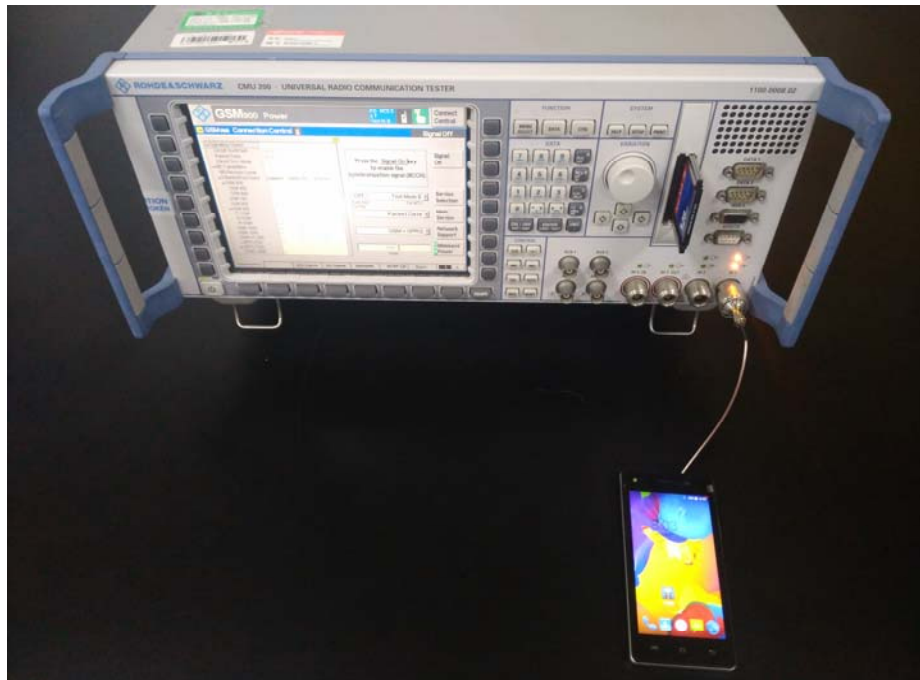
Photograph –2G&3G Conducted Test Setup
