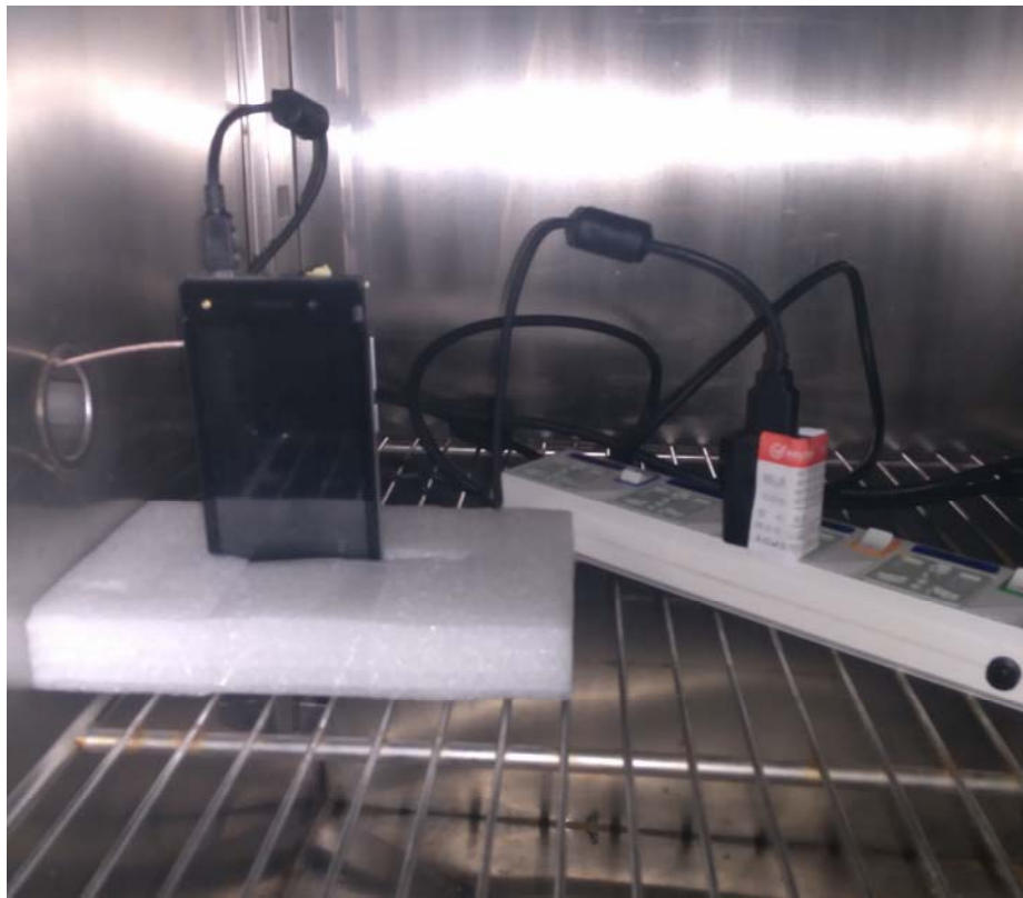
Photograph –2G&3G Conducted Test Setup
