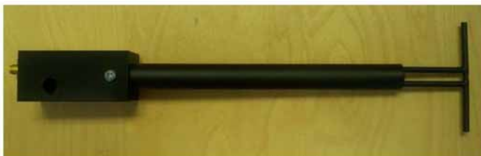
Figure 1 – MVG COMOSAR Validation Dipole
