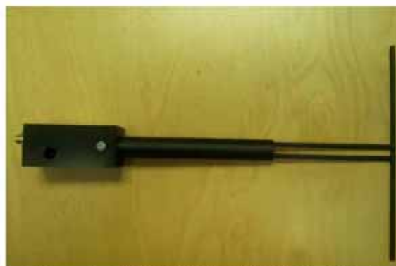
Figure 1 – MVG COMOSAR Validation Dipole
