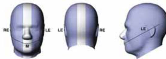
Figure 6.2 Front, back and side view of SAM
