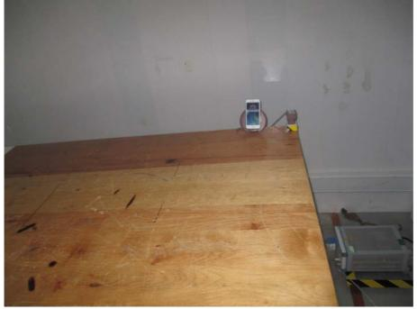
1.2 Radiated emission Test Setup
