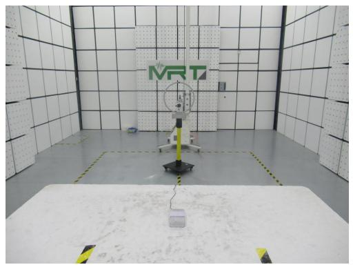
Test Mode: Mode 2 Description: Radiated Spurious Emission Test Setup for 30MHz ~ 1GHz
