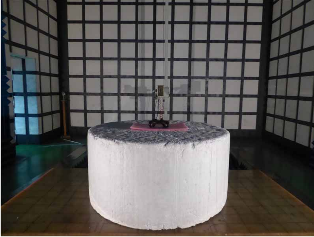
(In Anechoic 3m Chamber Test above 1GHz)
