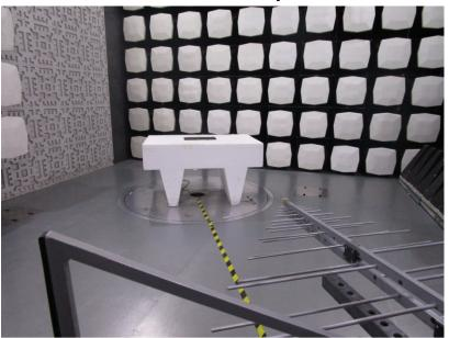
1.2 Radiated Spurious Emission Test Setup
