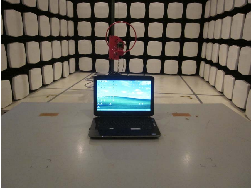
Measurement of Radiated Emission Test Set Up
