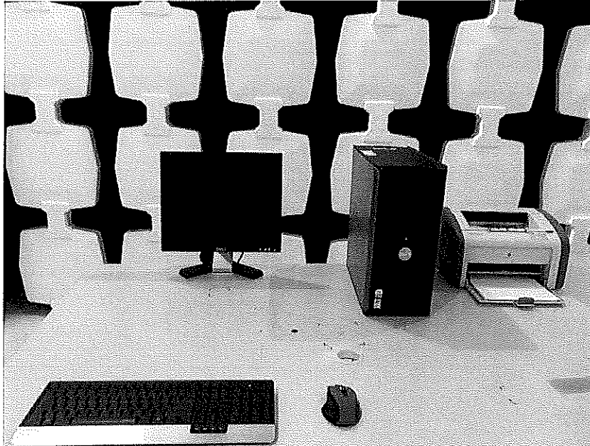
Measurement of Radiated Emission Test Set Up
