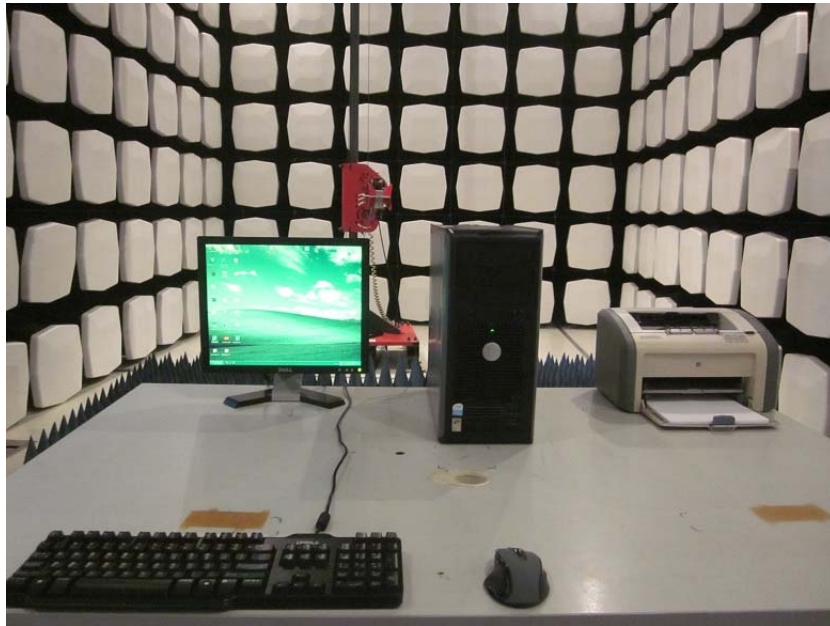
Measurement of Radiated Emission Test Set Up
