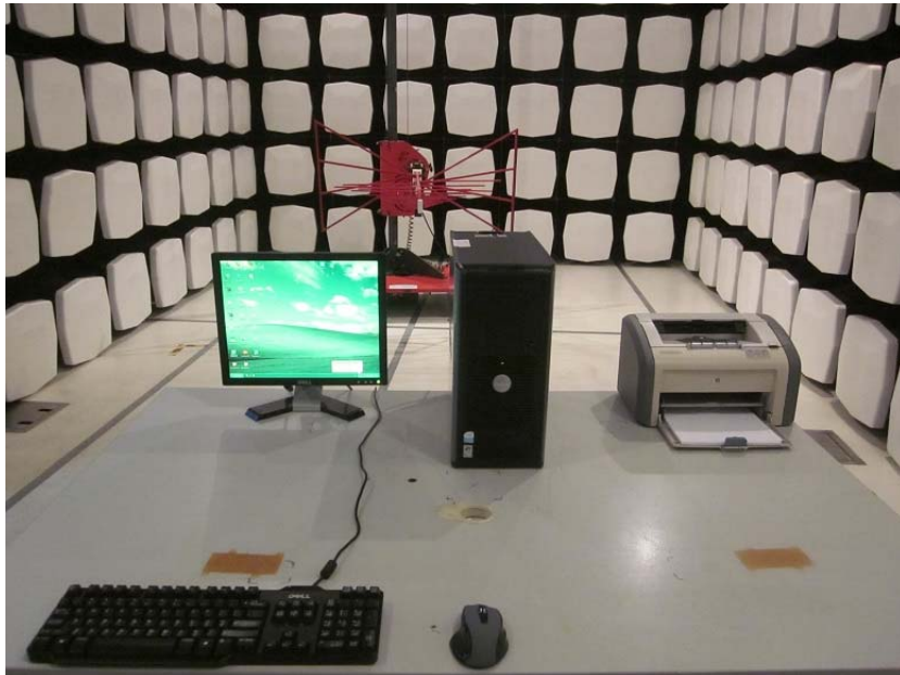
Measurement of Radiated Emission Test Set Up
