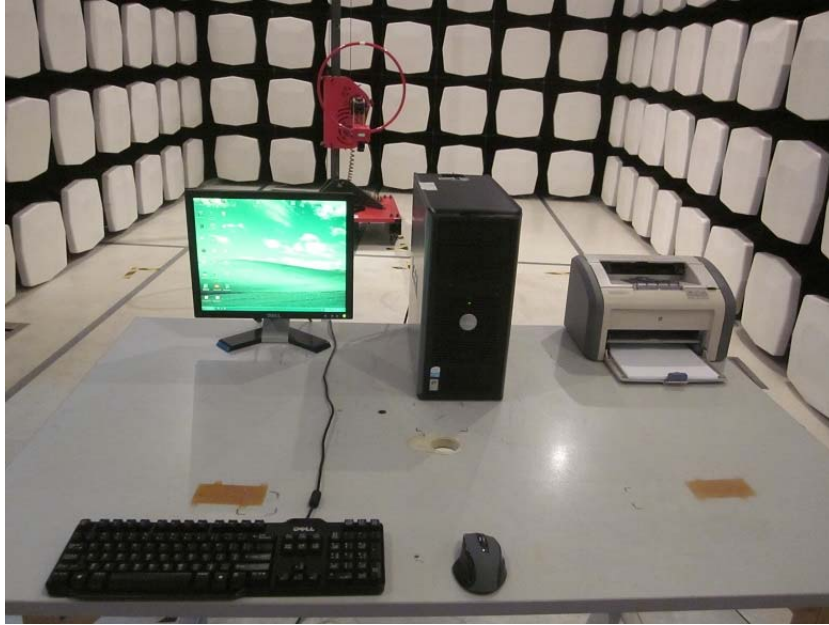
Measurement of Radiated Emission Test Set Up
