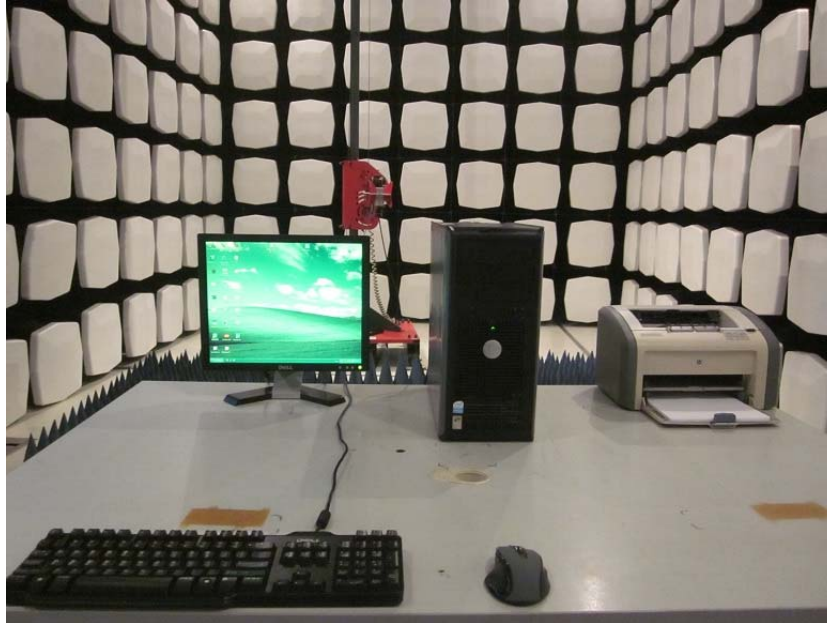
Measurement of Radiated Emission Test Set Up
