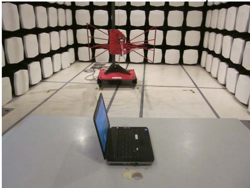
Measurement of Radiated Emission Test Set Up
