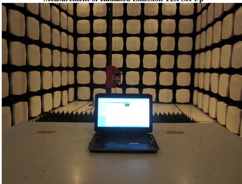
Measurement of Radiated Emission Test Set Up
