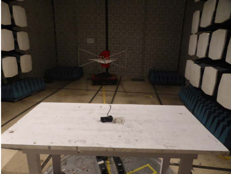
TEST SETUP OF RADIATED EMISSION (30MHz-1GHz)
