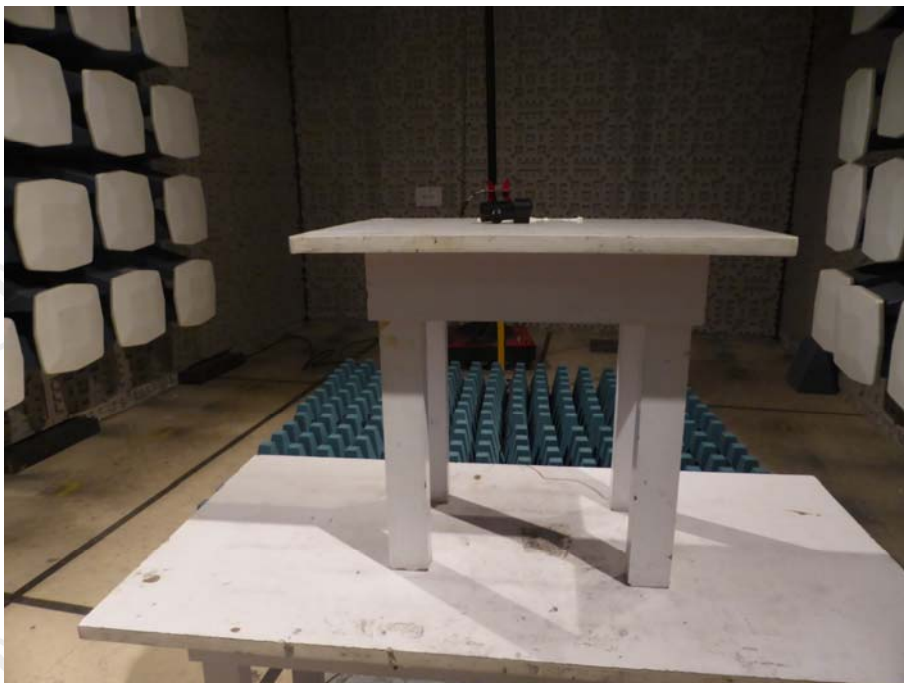
TEST SETUP OF RADIATED EMISSION (above 1GHz)
