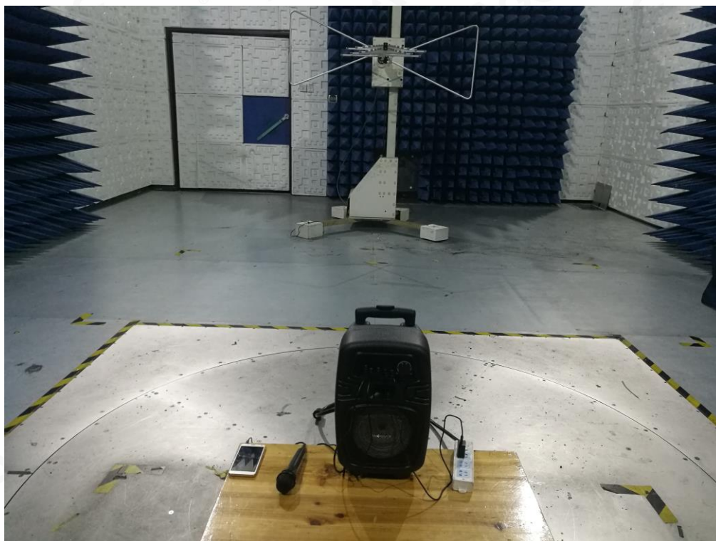
RADIATED EMISSION TEST SETUP ABOVE 1GHZ
