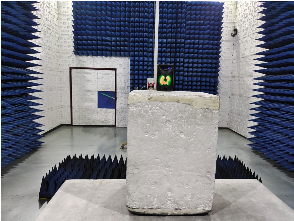
RADIATED EMISSION TEST SETUP ABOVE 1GHZ
