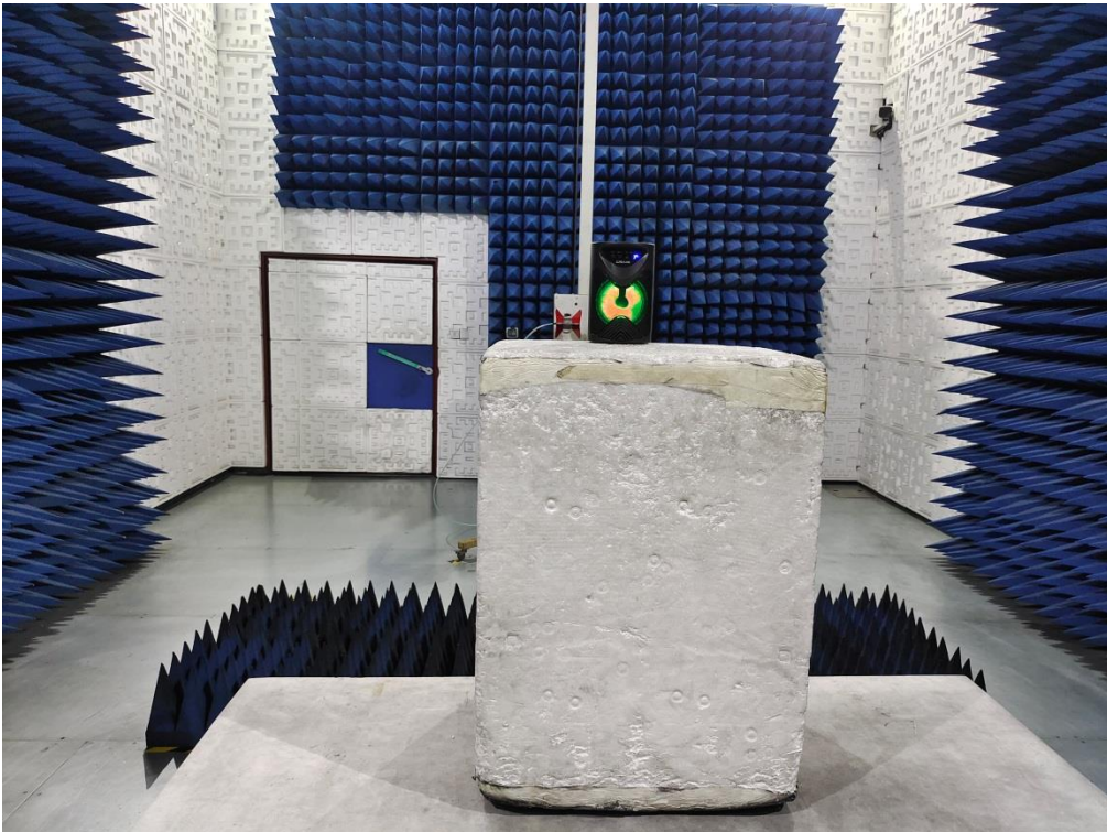
RADIATED EMISSION TEST SETUP ABOVE 1GHz
