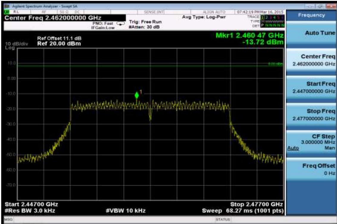
**802.11n\_HT40****Power Spectral Density Test Plot (CH-Low)**
