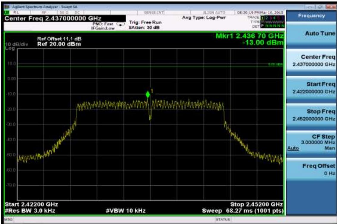
**Power Spectral Density Test Plot (CH-High)**
