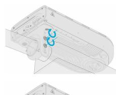
**B.** Then tighten the horizontal adjustment screws to 40 in-lbs torque using the 3/16" Hex bit driver.
