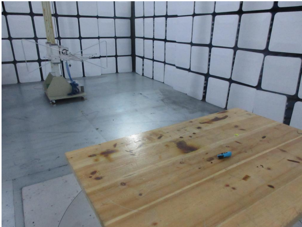
Photo of Radiation Emission Test
