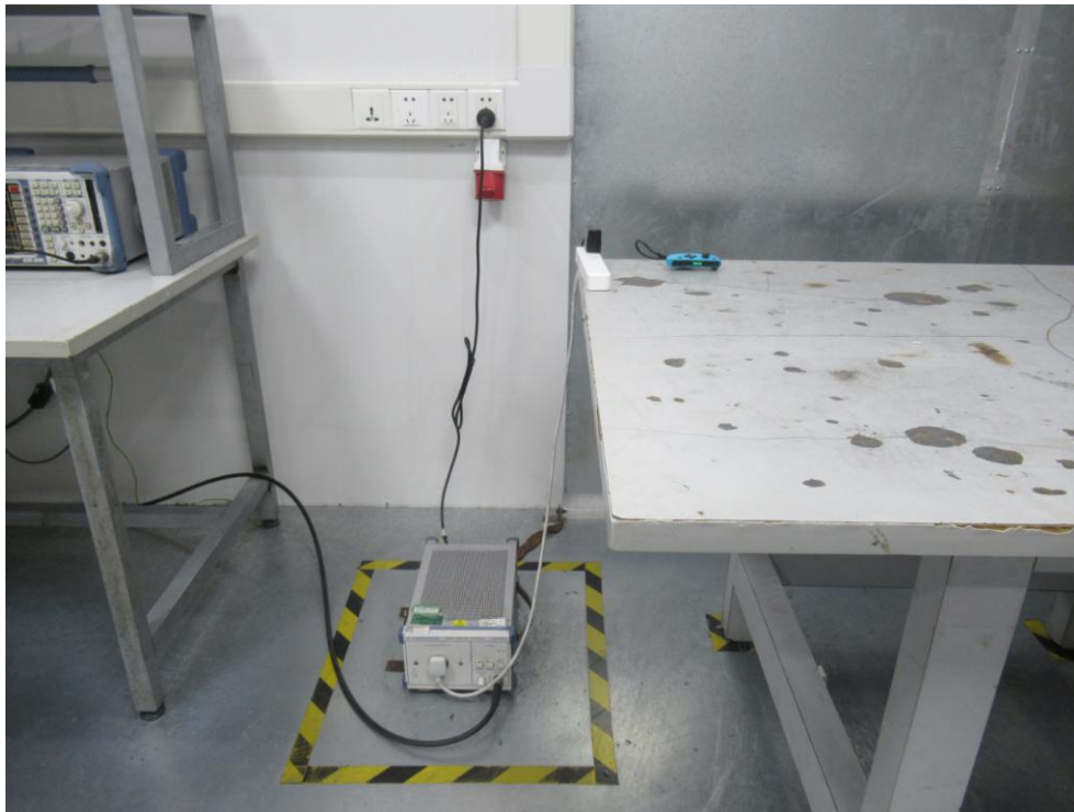
Photo of Radiation Emission Test
