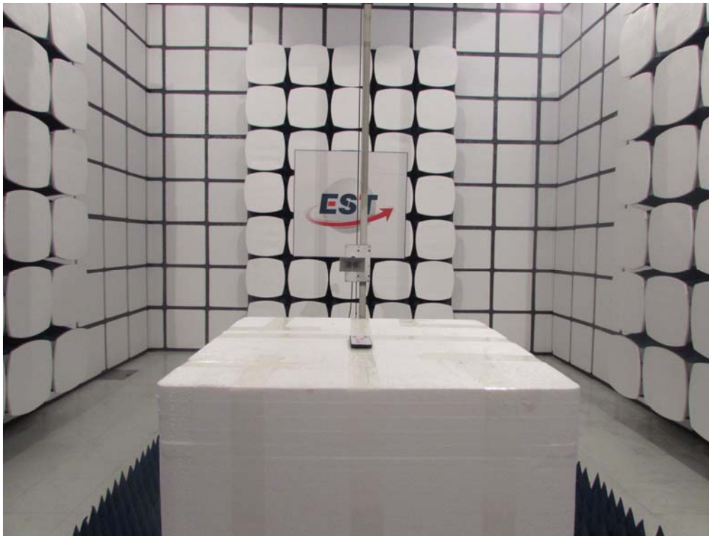
Set-up for radiated measurements (1000MHz to 5000MHz)
