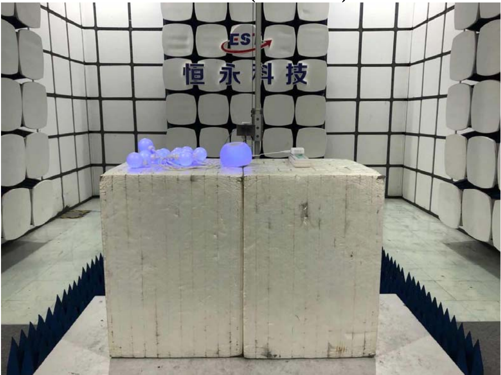
Radiated Test (Above 1GHz)
