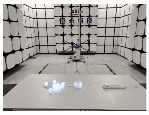
**Radiated Test (Above 1GHz)**
