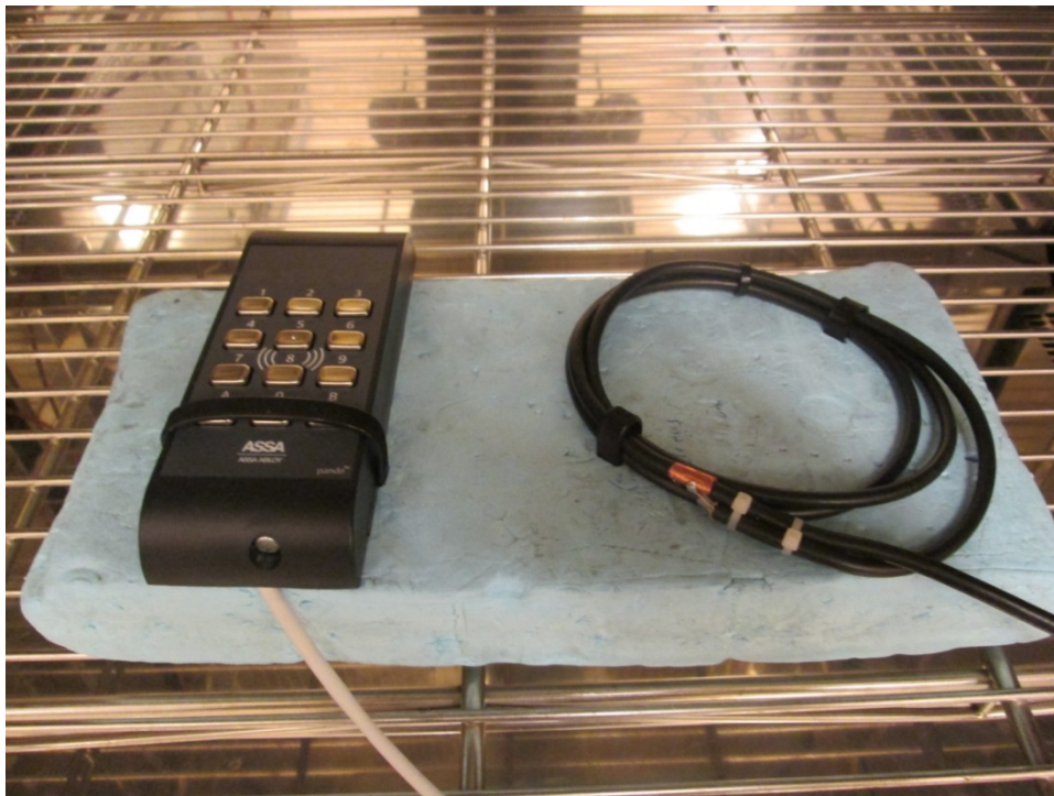
Photo 2.5.1 Test setup regarding test with extreme conditions with antenna and test object fixed mounted on a piece of polystyrene inside the climate chamber.
