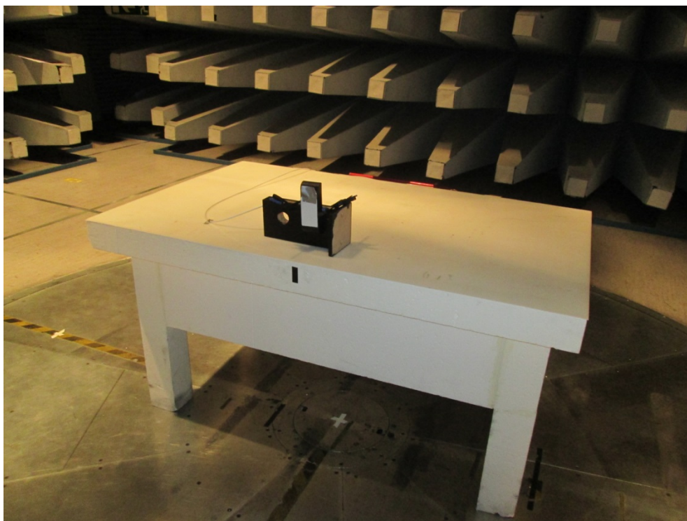
Photo 2.2.1 Test setup regarding measurement of radio frequency electromagnetic field.
