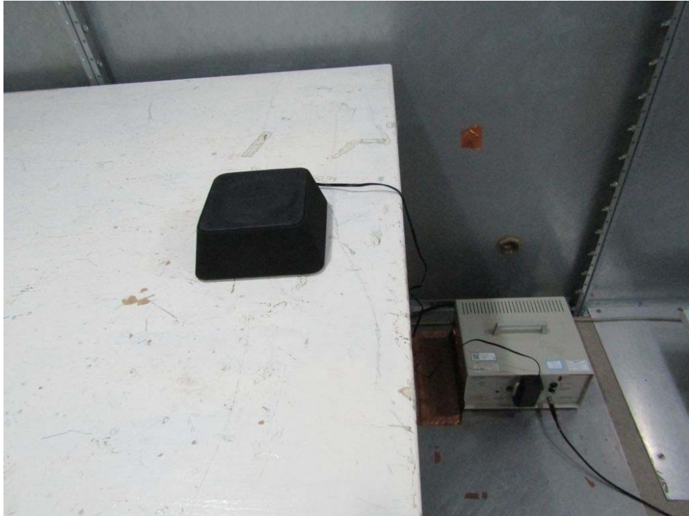
Measurement of Conducted Emission Test Set Up
