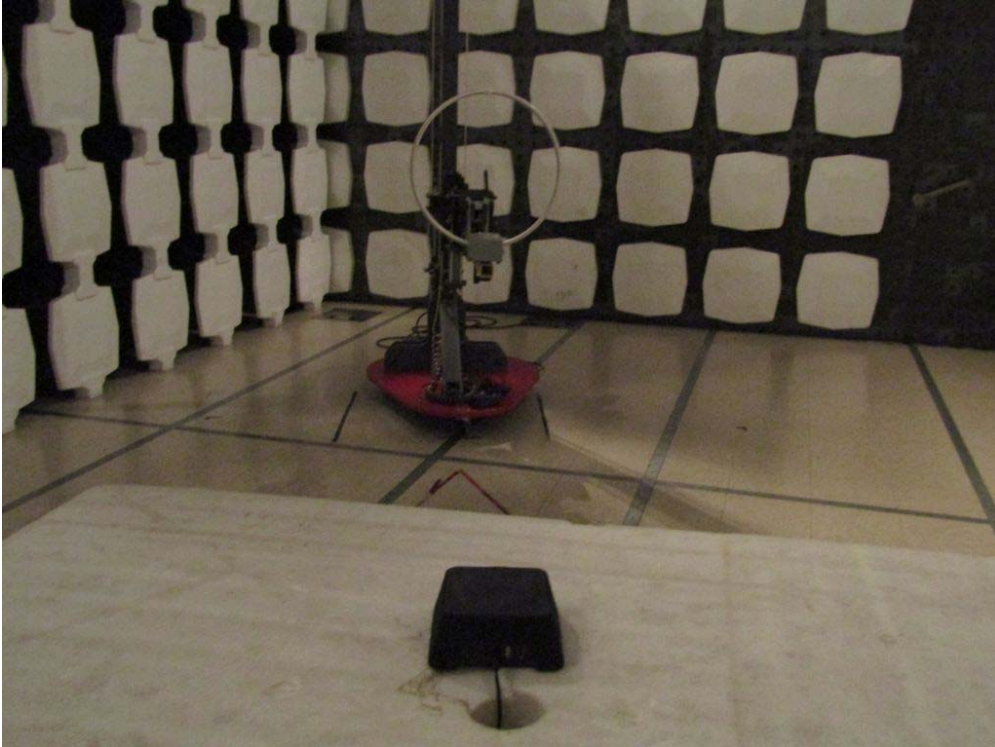
Measurement of Radiated Emission Test Set Up
